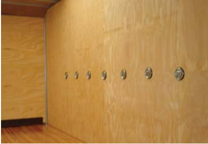
Full plywood lining and tie-down rings
